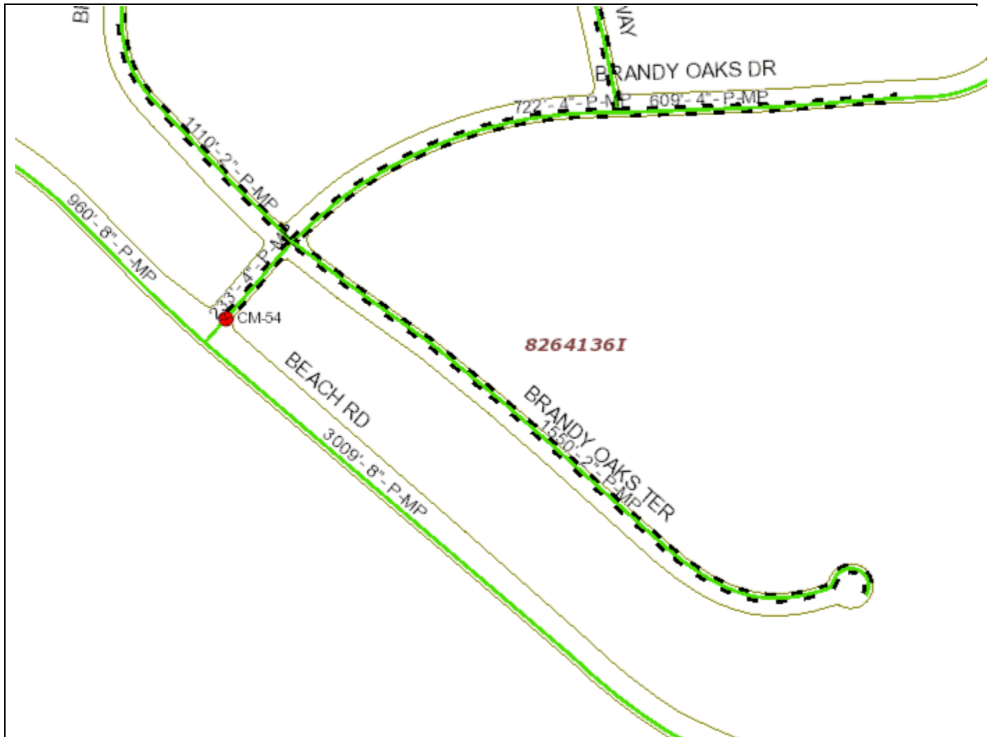
Propane Piping System Converted to Natural Gas: Normal Pressure Color Code Outlined with Black Dashes
