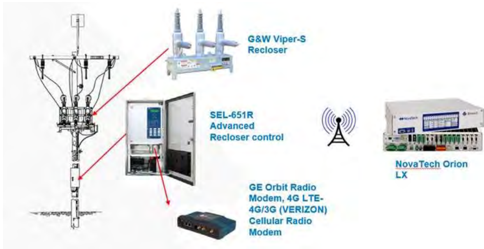
Figure 11. National Grid Pole-top Reclosers and Controls
