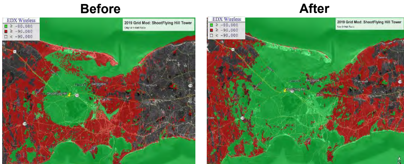
Figure 6. Maps Showing the Increased Coverage with the Addition of a Master Radio at Shoot Flying Hill
