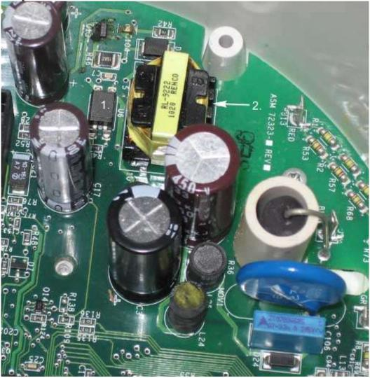
This shows the section of the circuit board that holds the power supply and surge protection components. The SMPS seems to be a fairly ordinary 12-volt DC one-amp power supply. The current waveform shown on page five indicates little was done to address power factor (discussed on p. 4).
