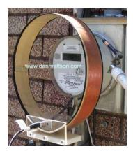
These are the two antennas I used for the measurement of the radiated emissions from the SMPS. I made the loop antenna about five years ago. It is about 12 inches in diameter and has about 120 feet of 18-gauge wire wrapped in a single layer. I had the opportunity to compare it to a high-end loop antenna. It compared well. I have no calibration data on it, but it works best as a 50-ohm antenna. It is usable from ELF to about one GHz. It is best from about 1MHz to 30 MHz.
