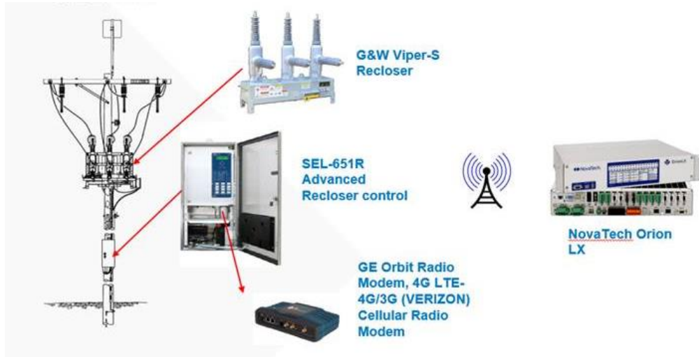
Figure 13. National Grid Pole-top Reclosers and Controls
