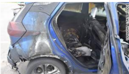
A 2019 Chevrolet Bolt EV parked in its owner's driveway in Vermont was charging when it caught fire. The fire has prompted one of the most expensive car recalls on record.
