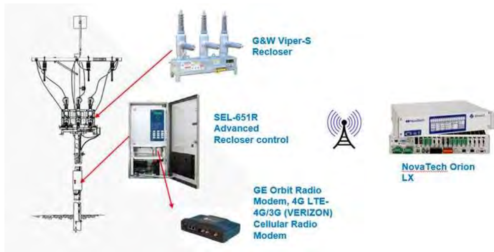
Figure 13. National Grid Pole-top Reclosers and Controls
