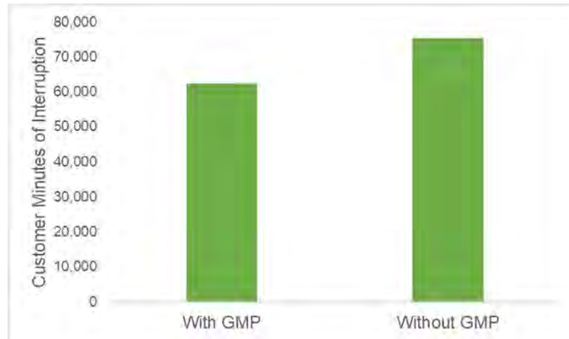
Figure 29: Savings in Customer Minutes of Interruption with GMP. 495 customers experienced an extended outage out of 2,845 customers on the circuit. Chart does not show benefit of non-GMP automation.
