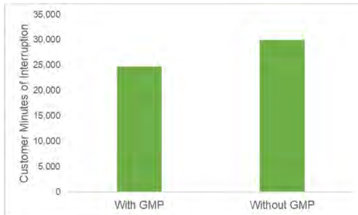
Figure 30: Savings in Customer Minutes of Interruption Due to Grid Modernization. 495 customers experienced an extended outage out of 2,845 customers on the circuit. Chart does not show benefit of non-GMP automation.
