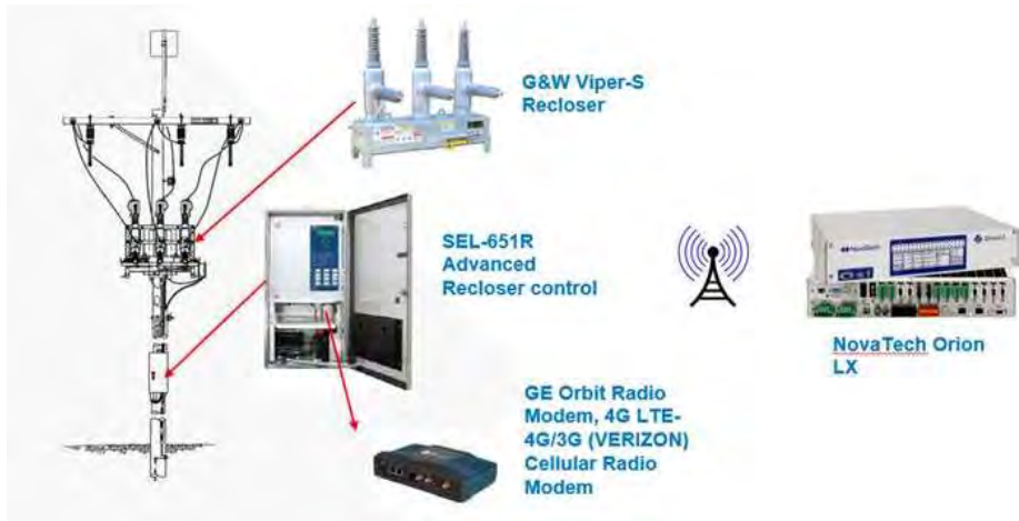
Figure 13. National Grid Pole-top Reclosers and Controls
