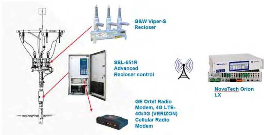
Figure 16. National Grid Pole-top Reclosers and Controls
