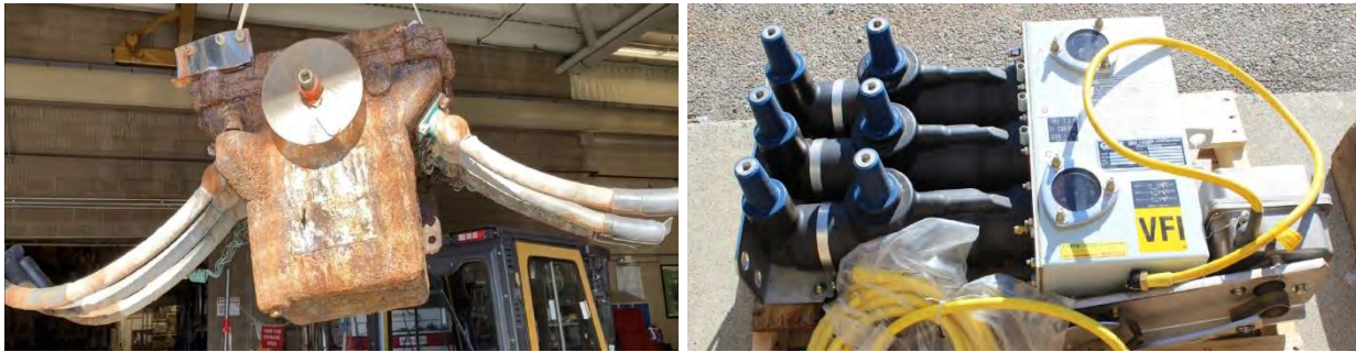
Figure 10. Old Oil-Filled Switches (Left) and New VFI Switches (Right)
