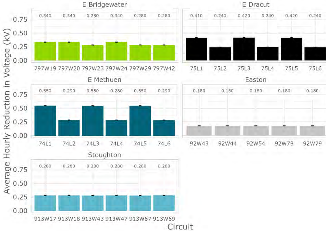
Figure 11. Average Hourly Voltage Reductions (kV) for National Grid VVO
