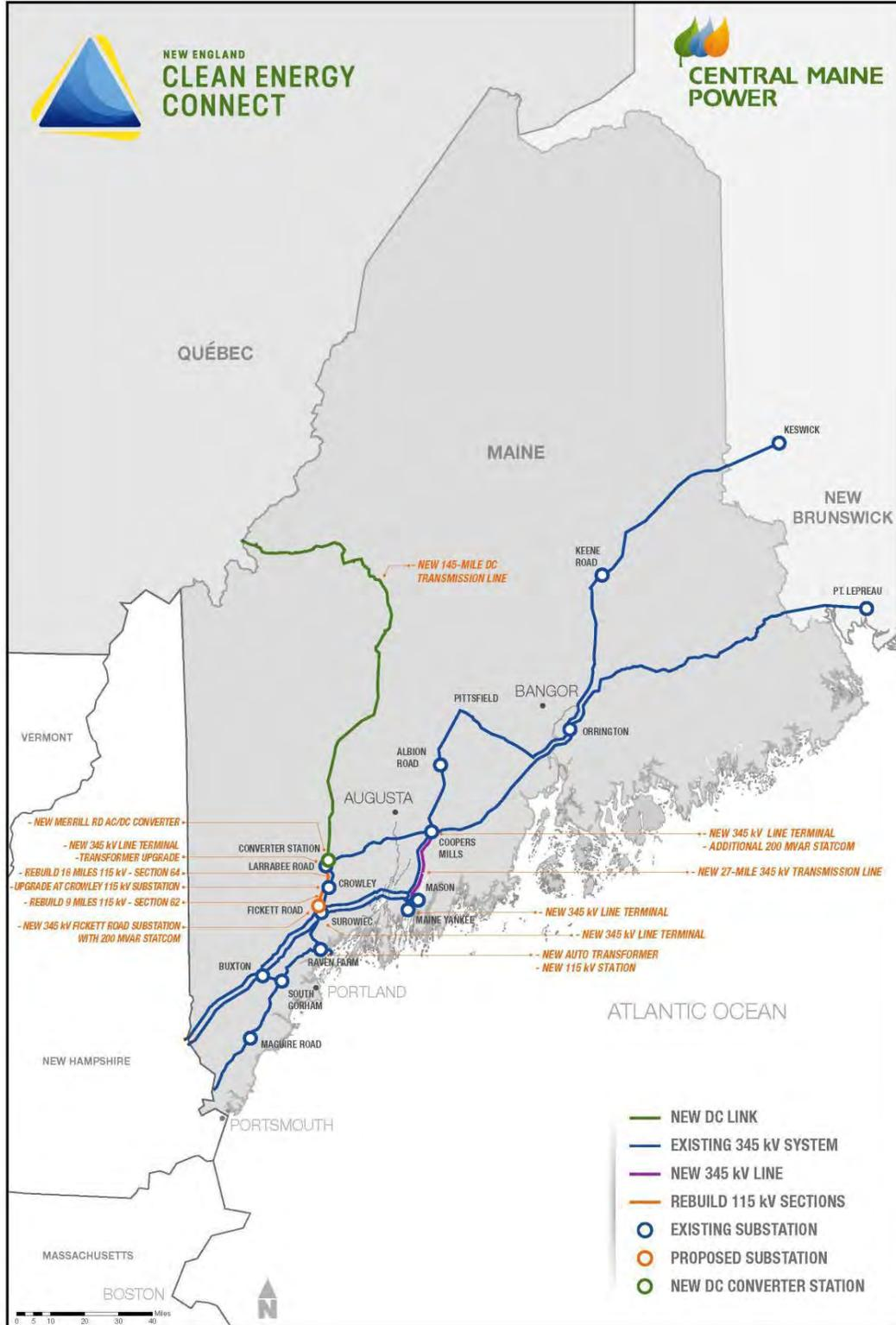
Figure 1 – Map Depicting the Components of the NECEC Transmission Line
